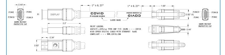
Active HDMI Cable - Ethernet - 28 AWG Plenum
