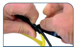
Secure mesh edge with tape, catching a small amount of the cable (approximately 1 inch).
