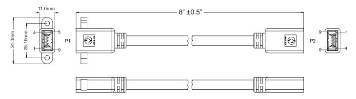
USB 3.2 Gen 1 Panel Mounted A Female to A Female Pigtail Cable
