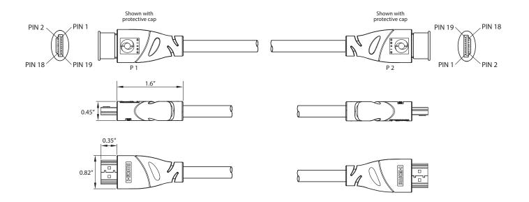
High Speed HDMI Cable Non-Plenum
