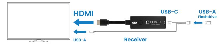
Note: Only connect the flashdrive once the RX is connected to the TV and is currently powered and showing up on screen.
