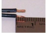
Unplug the power supply from the outlet first; cut off the original DC plug if using a non-Luxi power supply, separate the two wires for about 1" (2.5 cm) long, strip off the wire insulation precisely 3/16" (5 mm) from the end;
