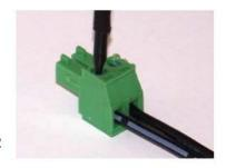
same location, one Luxi external power supply can power up to 5 units. Use extra insulated wires (18 AWG to 22 AWG) daisy-chain the multiple power input captive screw plugs, connecting all positive side together, and connecting all negative side together.
