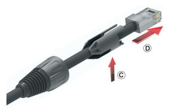
© Put the chuck onto the cable.
