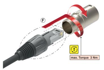
F Slide the unit (insert and boot) into the housing and tighten the bushing with max. torque 3 Nm (2.2 lb-ft).
