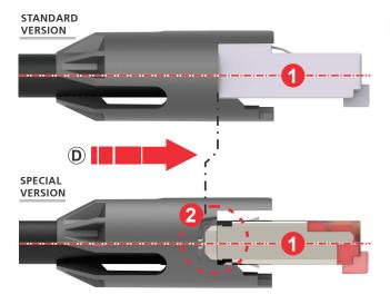
D Position the RJ45 in the chuck.
