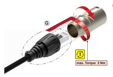
**G** Slide the unit (insert and boot) into the housing and tighten the bushing with max. torque 3 Nm (2.2 lb-ft).
