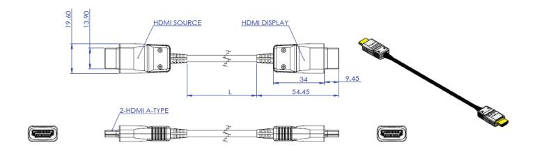
HDMI Shielded AOC Cable Plenum
