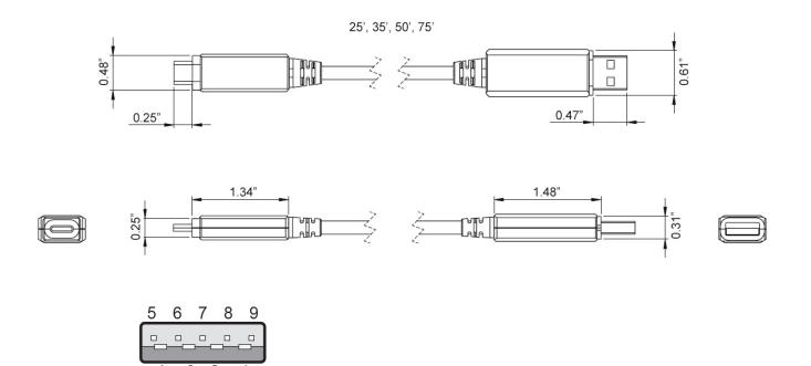
USB 3.2 Gen 2 Active Optical Cable Plenum
