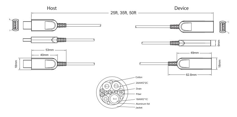
USB 3.2 Gen 2 Active Optical Cable Plenum
