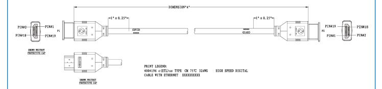
HDMI 2.0 Cable - 18G - Slim Line - 32 AWG Non-Plenum
